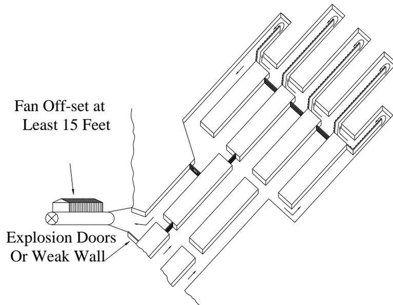
Air circulates through a mine because there is a difference in pressure between the intake and the return. The difference in pressure can be created by the difference in temperature, elevation, or by mechanical means. See illustrations. Natural ventilation isn't reliable because the direction, of the air current, may reverse with weather conditions, and when the outside temperature approximates the inside temperature, movement of air will cease.
