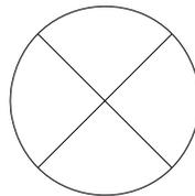
Regulator - An adjustable door or opening in a stopping generally placed across a return airway, and used to adjust the amount of air passing through the airway in order to properly distribute airflow.
