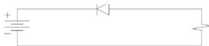
b) Reverse Bias - Current is not conducted.
