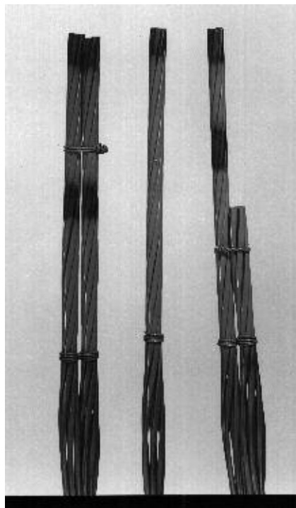
Single and double birdcaged bolts (photograph courtesy of ANI Arnall)
