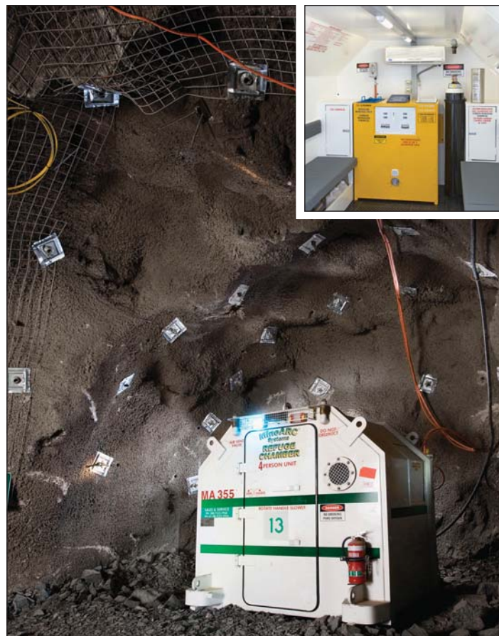
A hard-rock refuge chamber, identical to that which was used in yesterday's at Leinster's underground rockfall. Top right: Inside the refuge chamber.
