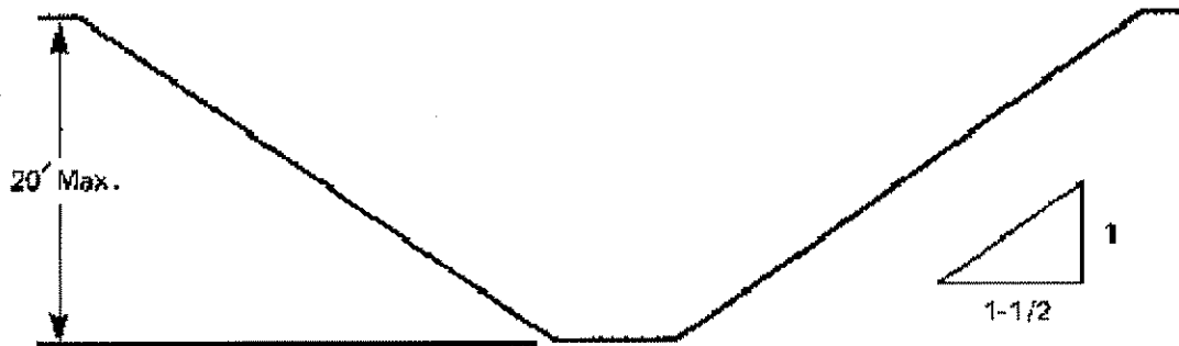
Figure 1. Excavations Made in Type C Soil All simple slope excavations 20 feet or less in depth shall have a maximum allowable slope of 1 1/2:1.
