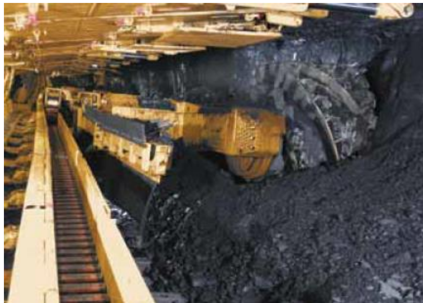
Figure 67. Installed CAT longwall system, showing the shearer. (Grayson, 2014)
