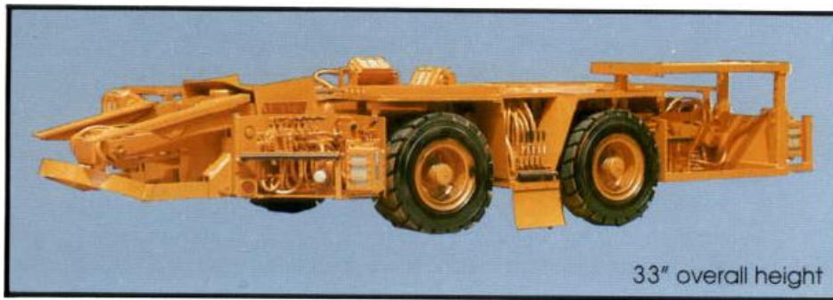
Figure 46. A picture of a single-beam roof bolting machine (J.H. Fletcher & Company, 2015).
