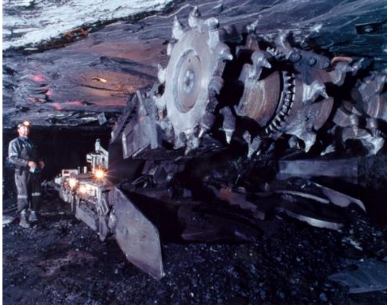
Figure 4. Picture of a continuous mining section in action (Coal Leader, 2015).
