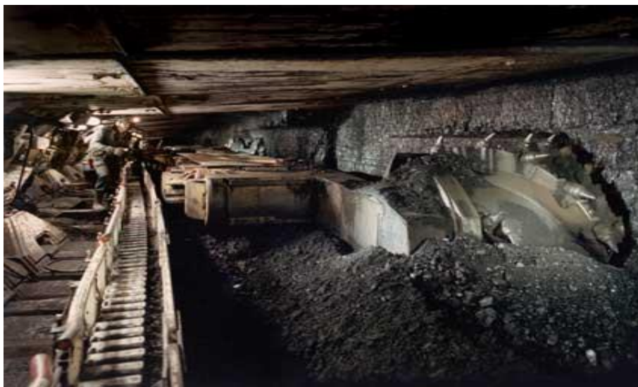
Figure 6. Picture of a longwall face being mined (Grayson, 2014TABLE OF CONTENTS
