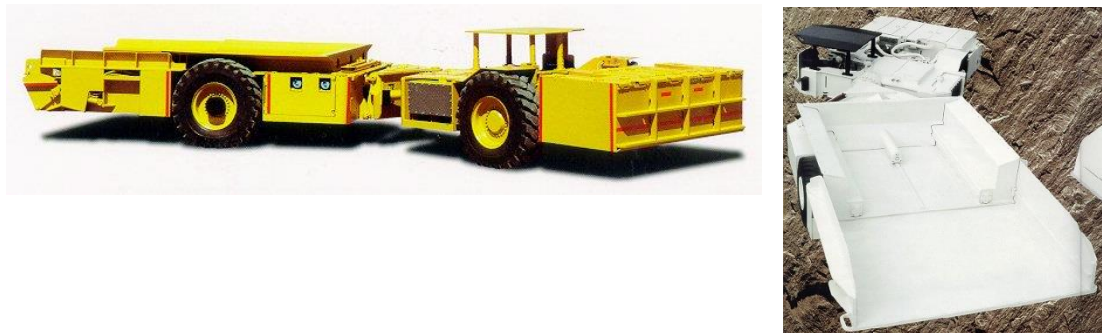
Figure 38. Two articulated battery-powered models of face haulage vehicles (Grayson, 2014).
