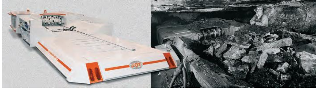
Figure 47. An example Stamler feeder-breaker (Joy Global Inc., 2015).
