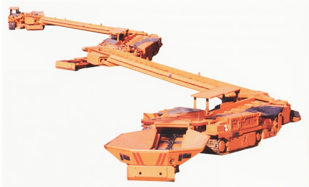
Figure 40. A second type of continuous haulage system with a chain conveyor. (Joy Global, Inc., 2015)
