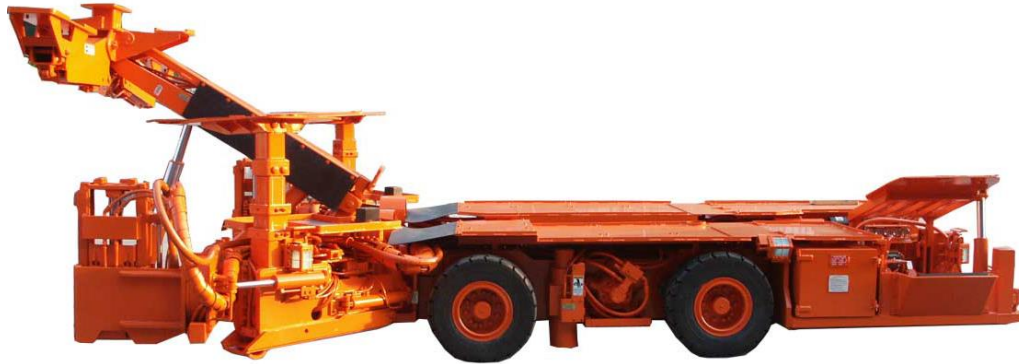
Figure 45. A picture of a dual-boom, H-beam type roof bolting machine (J.H. Fletcher & Company, 2015).
