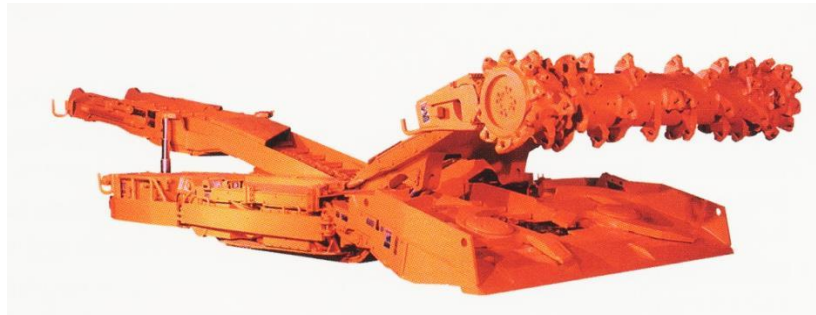
Figure 32. A Joy Global Inc. continuous mining machine. (Joy Global, Inc., 2015)
