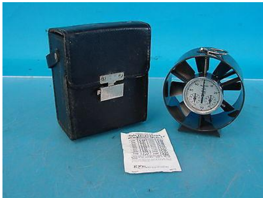
Figure MV-41: Taylor Anemometer with Case and Calibration Sheet
