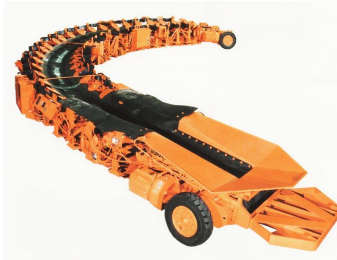
Figure 39. One type of continuous haulage system with a flexible belt. (Joy Global, Inc., 2015)
