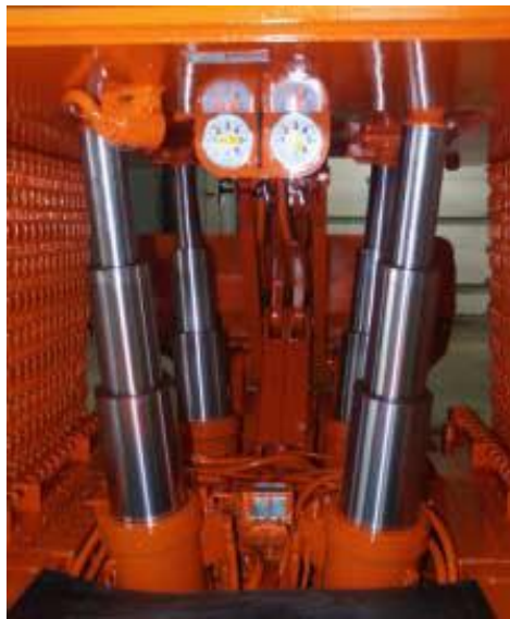
Figure 43. Side and front pictures of a pre-implementation mobile roof support.
