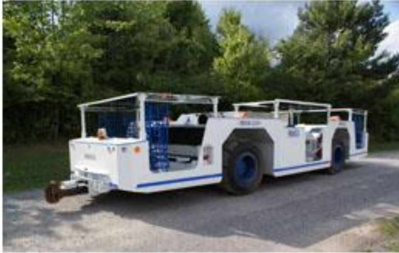
Figure 49. Diesel mantrip/personnel carrier (Brookville, 2015).
