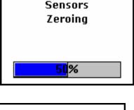
If the user selects OK, all the installed sensors are zeroed first (following the Zero All steps) and then calibrated. After the zero, the results are shown, for 5 seconds and then the calibration of the first sensor begins.
