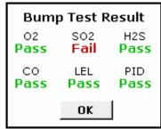
If there is more than one sensor that failed the bump test, they are calibrated in order (top row left to right, bottom row left to right on the Normal Readings screen), one at a time – each time prompting the user to choose whether to calibrate the sensor or not.
