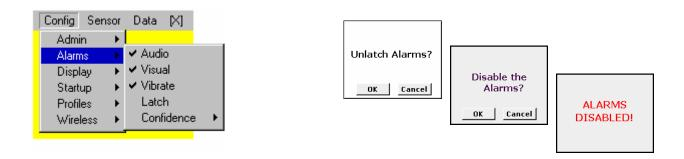
If all 3 alarms are disabled, "ALARMS OFF!" is displayed on the bottom of the NRS in red.
