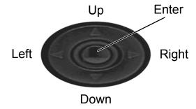
To shut down the instrument, hold the center [ENTER] navigation button for more then two seconds. A confirmation screen is displayed to provide verification of the shut down.
