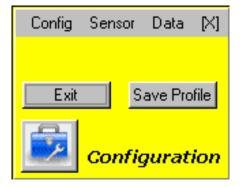
The Exit Button and the [×] exits Configuration mode and returns to the Normal Readings screen. Changes to the configuration are saved while the instrument remains on, but do not affect the current profile.
