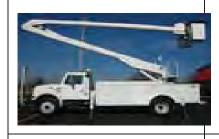
**Vehicle Mounted Aerial Lift / Bucket Truck** The lift platform is an integral part of an over the road vehicle.
