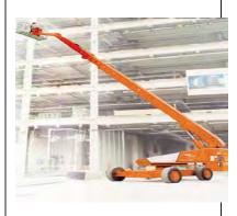
**Extendable / Telescoping Aerial Lift** This aerial lift has a boom that extends horizontally and vertically.
