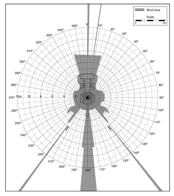
Blind Area Diagram for Construction Vehicle – 900 mm Plane
