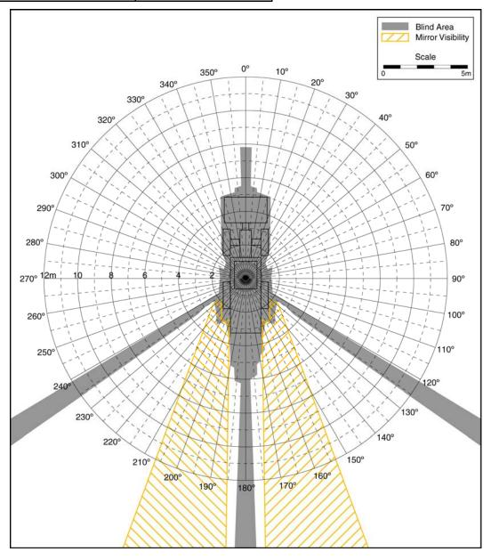
Blind Area Diagram for Construction Vehicle – Ground Plane
