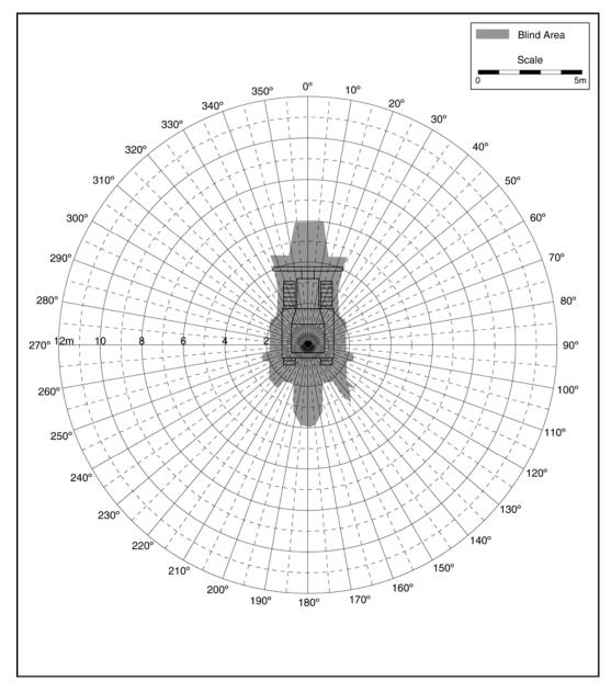
Blind Area Diagram for Construction Machine – 1500 mm Plane
