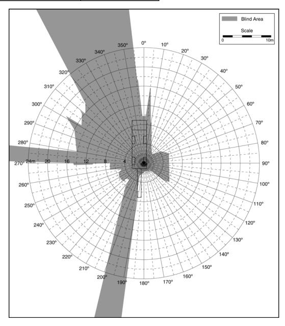
Blind Area Diagram for Construction Vehicle – 1500 mm Plane
