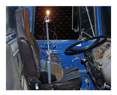
Figure 3. Light Support Device Test Setup.
