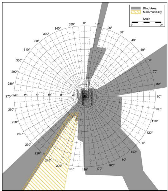
Blind Area Diagram for Construction Machine – 900 mm Plane
