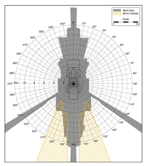
Blind Area Diagram for Construction Vehicle – 900 mm Plane
