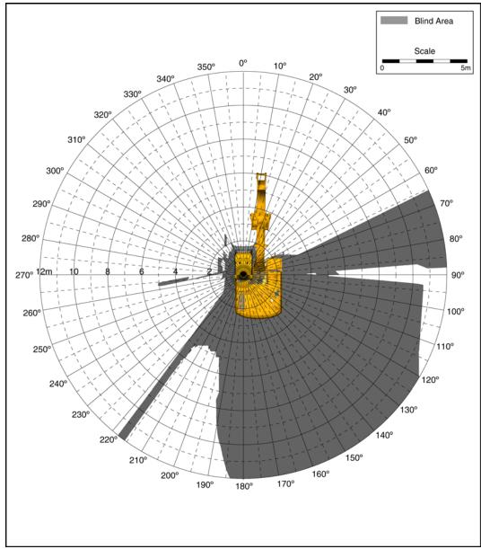
Blind Area Diagram for Construction Vehicle – 1500 mm
