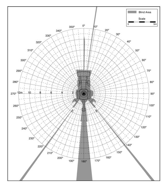
Blind Area Diagram for Construction Vehicle – 1500 mm Plane
