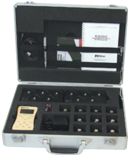
The doseBadge is often supplied as a complete measurement kit which includes all of the component parts needed to operate the system. This includes the doseBadge Reader unit, cables, power supply, charger, manuals and software.
