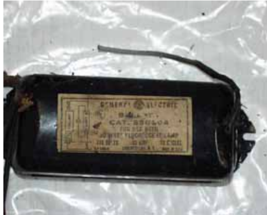
Fig. 4 Fluorescent light ballast
