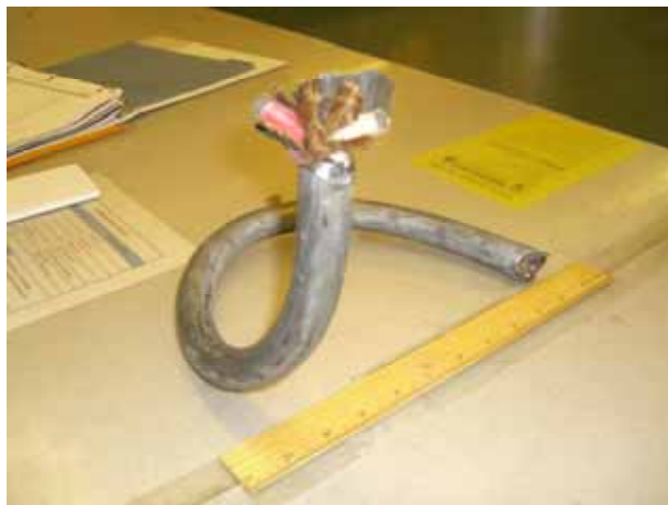
Fig. 5 Lead jacket electrical cable
