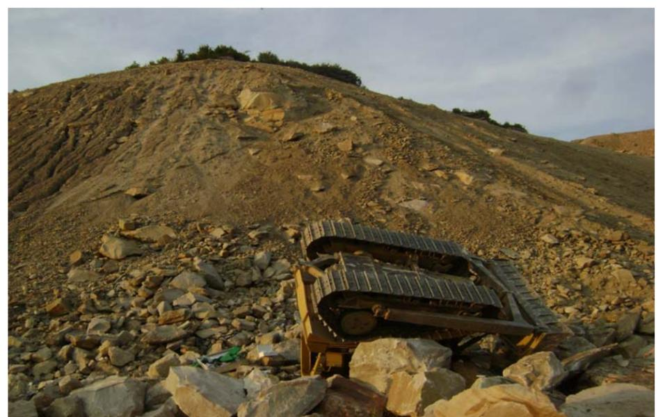
On September 19, 2008, a dozer operator was killed when the dozer he was operating flipped over and rolled approximately 180 feet down a slope. (See the Picture Above)
