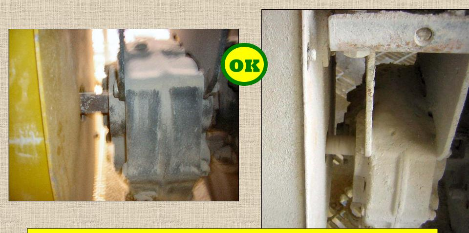
Smooth shafts – guards not required due to location and short length of smooth shaft exposed
