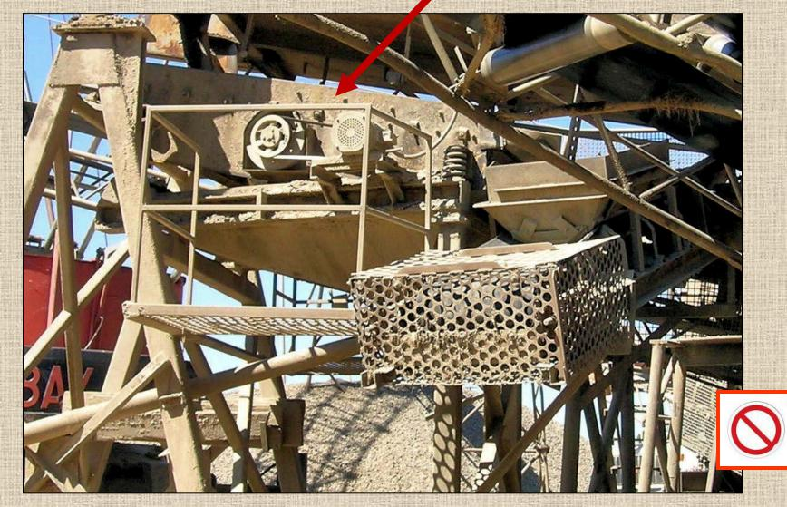
from MSHA's 2004 "Guide to Equipment Guarding" Handbook An area guard is a barrier which prevents entry of a miner into an area containing moving machine parts, thus preventing contact with the moving parts. Effective area guards may require additional practices and provisions, such as signage, locks, color coding, etc., in addition to the physical barrier. When designing, installing, and/or using area guards, consider:
