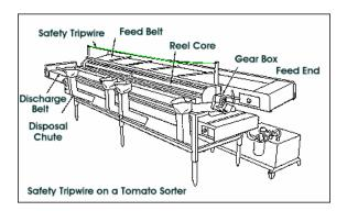
Safety **tripwire cables** may also be located around the perimeter or near the danger area.
