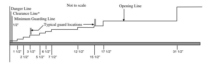
\*Guard must extend from some point on the clearance line to some point on opening line
