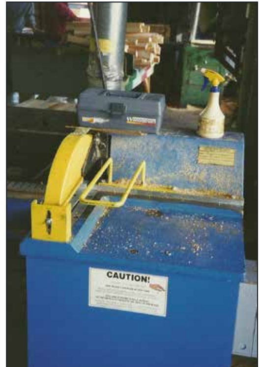
Properly guarded jump saw.
