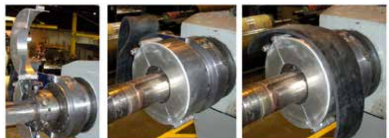
Fabricated quill-mounted guard to enclose cathead.
