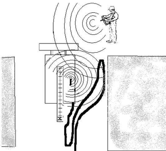
If the remote control continuous miner is not following the commands of the radio remote control, DO NOT get within the machine's turning radius to get closer to the machine's antenna.
