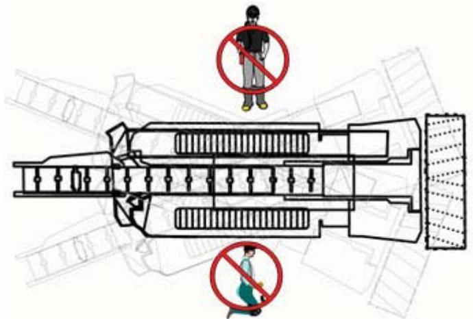
The middle of the remote control continuous miner (pivot point) is not a safe place from which to reposition or tram the machine during a place change.
