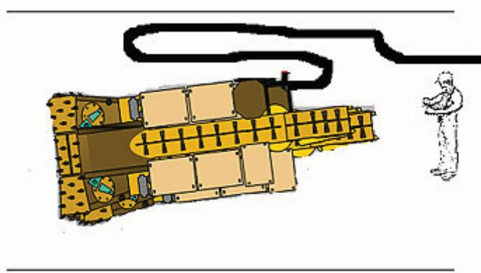
When handling the cable within the turning radius of the remote control continuous miner, de-energize the machine and remote control unit according to established safe work practices.
