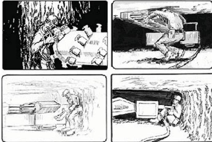
Fatal accident statistics show that the majority of all non-maintenance related crushing accidents involving remote controlled continuous mining machines happened when the victim was located within the turning radius of the machine while it was being trammed.
