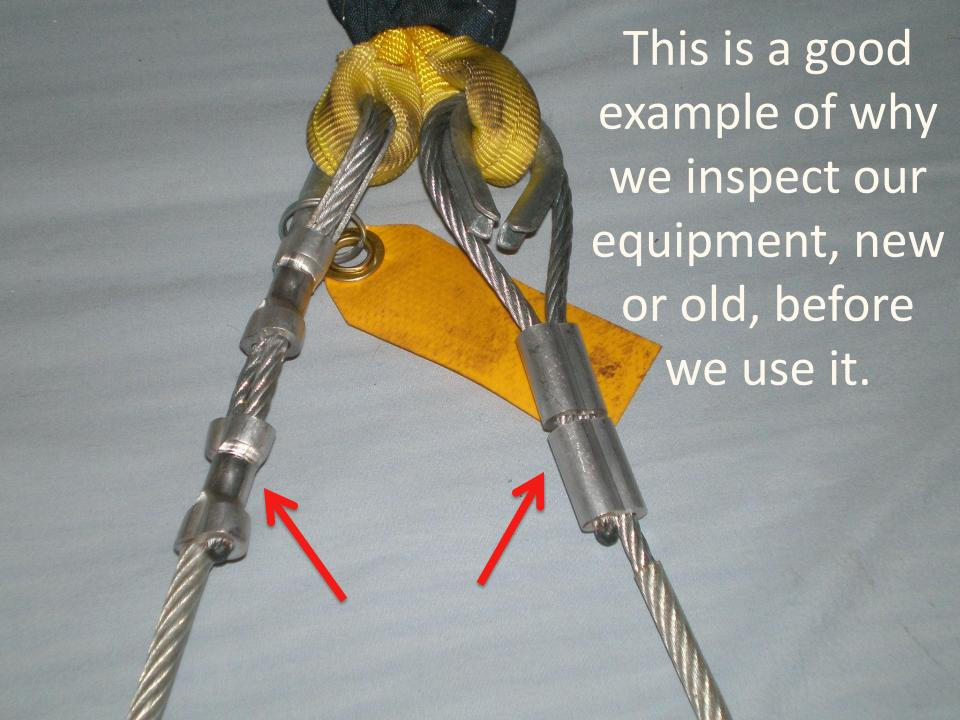
The lanyard was taken from the store, in a new package and was never used. You can see where all the connections are crimped – except the 2 for the one lead (see arrows)
