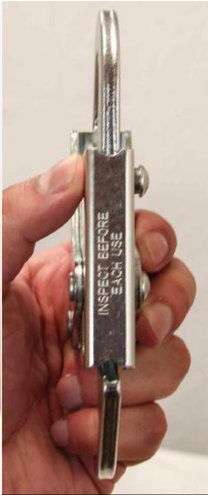
Figure 6A: Attempt with pressure to unseat rivet
