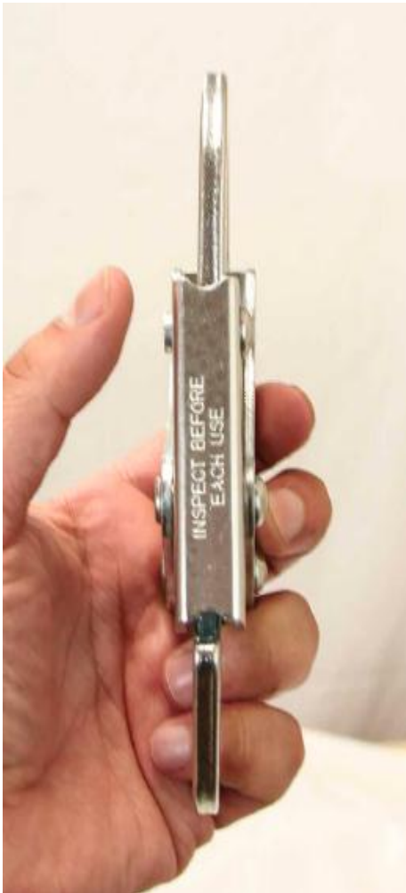
Figure 6: Turn hook to side and push "Tail" end of rivets with thumb or finger
