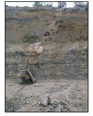
On September 16, 2013, a 58-year old truck driver with 25 years of experience was killed at a crushed stone operation. The victim was driving a loaded haul truck out of a quarry when the truck traveled through a berm and over an 80-foot highwall. The victim was ejected from the truck.
