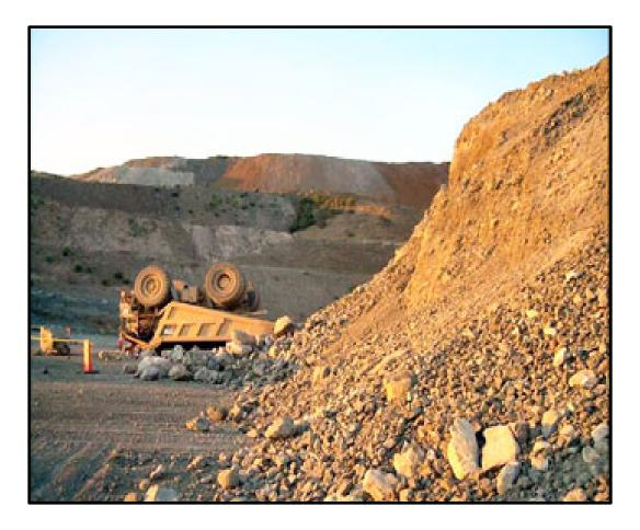
On May 27, 2008, a 52-year old truck driver with 2 years experience was fatally injured at a surface crushed stone mine. The victim backed a truck to the edge of a stockpile to dump. The truck went over the crest and fell approximately 30 feet to the floor below.
