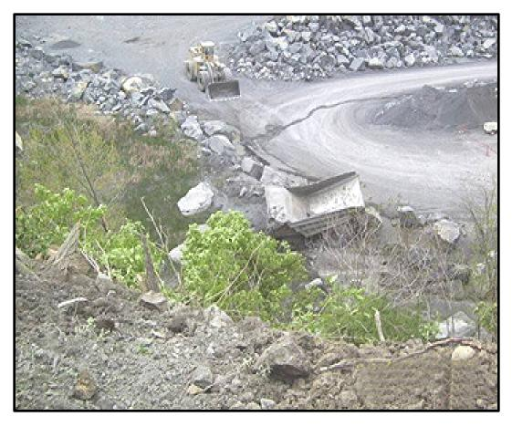
On April 25, 2007, a 65 year-old truck driver, with 42 years mining experience, was fatally injured at a cement operation. The victim was operating a haul truck that veered off the roadway, climbed a berm, and fell over a highwall onto a bench below. The victim was not wearing a seat belt at the time of the accident and was ejected from the cab of the truck.
