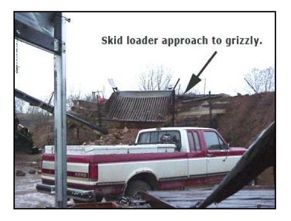
On April 4, 2005, a 47-year-old laborer, with eight days mining experience, was fatally injured at a surface sand and gravel operation. He was operating a skid loader and dumping material into the plant grizzly. The loader traveled onto the grizzly; overturned, and landed on the ground below. The victim, who was not wearing the seat belt, was ejected.
