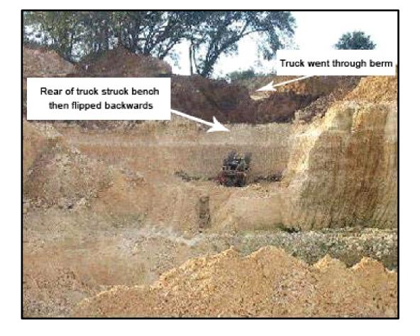
On November 4, 2005, a 21-year old laborer with 5 weeks mining experience was fatally injured at a crushed stone operation. The victim was being task trained to operate a haul truck. While backing down a ramp, he lost control of the truck. The truck went through a berm, overturned, and fell to the bench below.
