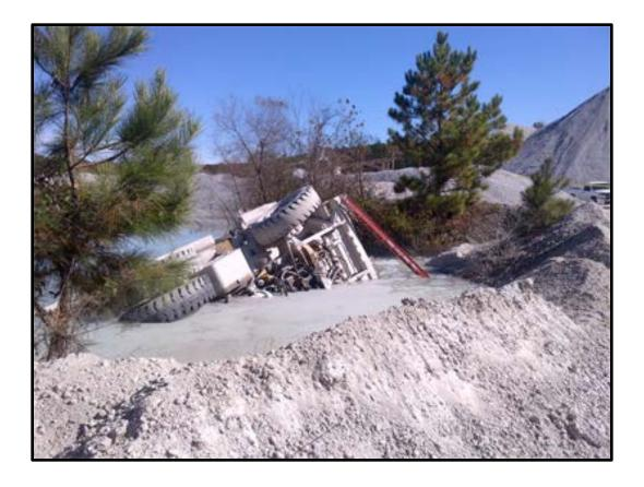
On November 7, 2013, a 46-year old equipment operator with 27 years of experience was killed at a granite mine. The victim was operating a haul truck when it veered off the left side of a haul road and traveled through a berm. The haul truck went over an embankment and overturned in a settling pond.
