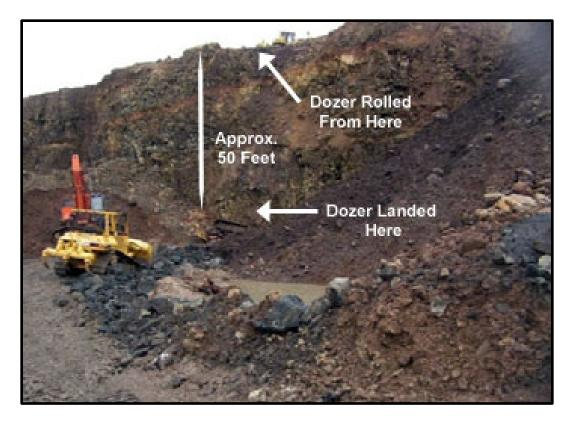
On January 27, 2006, a 60-year old heavy equipment operator with 10 years mining experience was fatally injured at a crushed stone operation. He was operating a dozer to prepare a bench for drilling. The dozer traveled over the edge of a 50-foot highwall and fell to the quarry floor, submerging the cab in several feet of mud and water.
