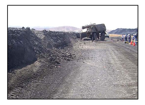
On July 30, 2005, a 23-year old contractor equipment operator, with 20 months mining experience, was fatally injured at a surface gold mine. The victim was operating a water truck that left the roadway and climbed the berm, causing it to overturn and land back on the haul road. The victim, who was not wearing a seat belt, was ejected from the cab of the truck.
