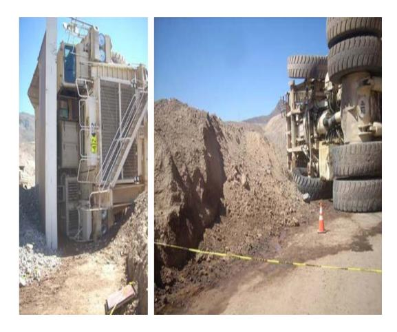
On September 27, 2009, a 28 year-old truck driver with 2 years of experience was fatally injured at a copper operation. He was operating a 240-ton haul truck that left the haul road and climbed a berm, causing it to overturn and land on the haul road. The victim, who was not wearing a seat belt, fell from the cab of the truck.
