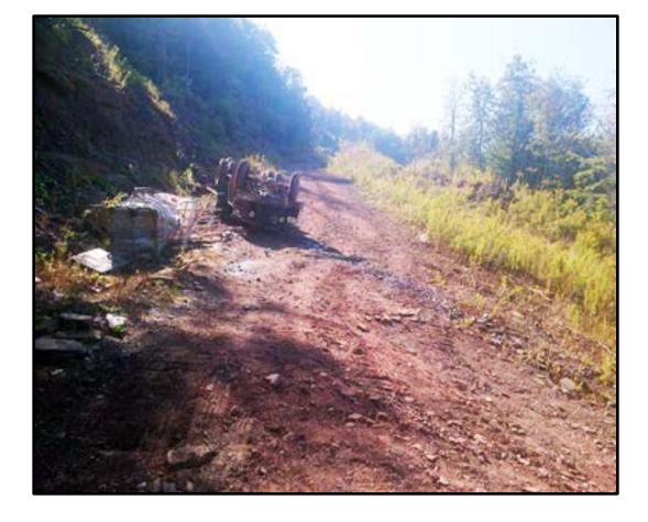
On September 19, 2013, a 32-year old laborer with 14 years of experience was killed at a dimension stone operation. The victim was operating a 2½ ton truck up a steep roadway. He was hauling water tanks in the bed of the truck when the load shifted and the truck overturned, crushing him.
