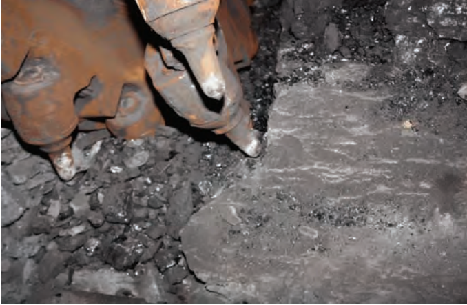
Photo 1. The longwall taildrum bits in a cut-out at the tail. The UMWA believes sparking from this area caused an initial methane ignition, which then grew into a coal dust explosion.
