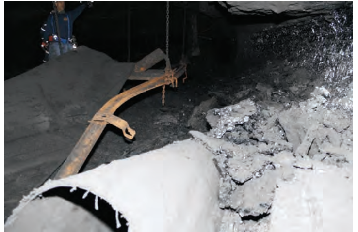
Photo 4. Bent and twisted steel belt structure at #4 crosscut of Tailgate 22 Section shows evidence from the forces of the explosion.
