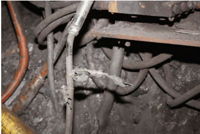
Melted canvas and plastic ties on air hose where canvas was used to direct airflow onto methane sensor on the longwall.
