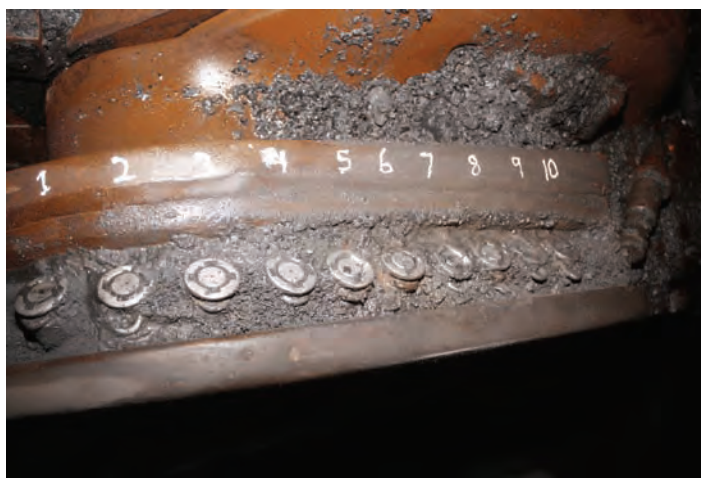
Headgate ranging arm sprays on the UBB longwall. Five of the ten sprays were plugged and did not work.
