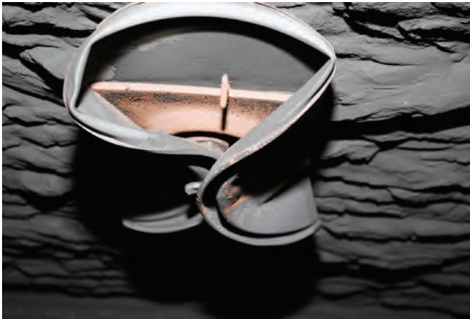
Roof bolt plate bent from initial path (left side) and secondary path (right side) of explosion.
