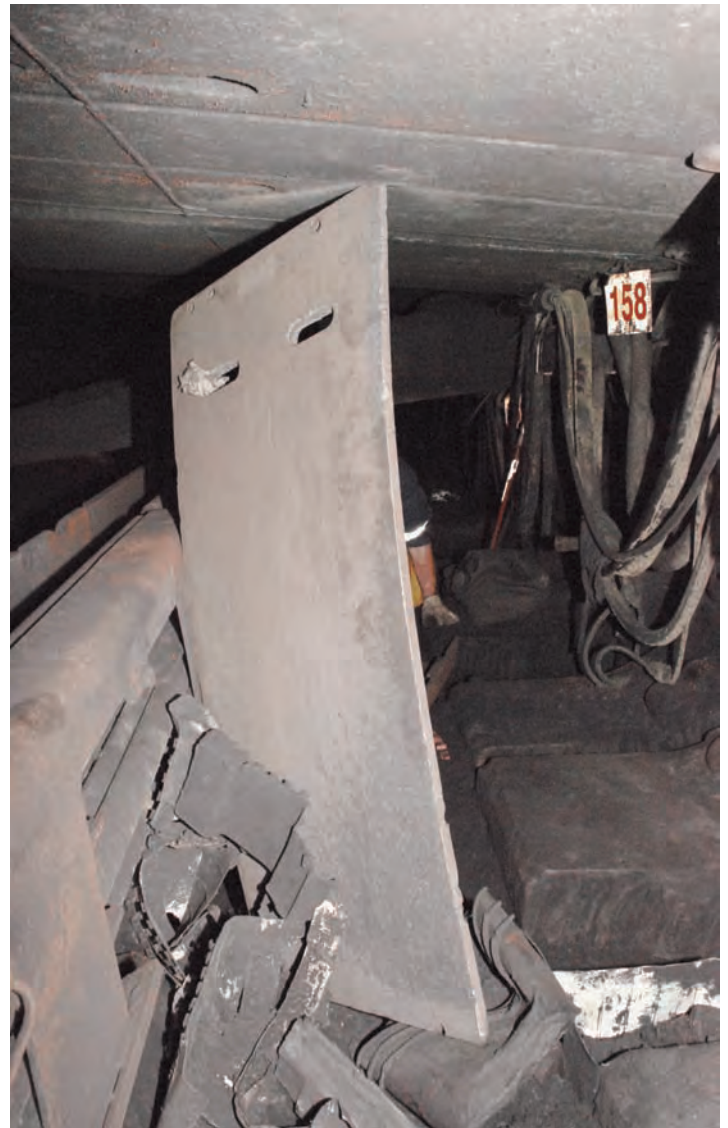
Photo 10. Tail drive assembly lid wedged between top of longwall shield and toes of shield at Shield #158.
