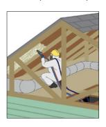
under the new standard. For instance, working in an attic and applying a large amount of spray foam (or another chemical) in a short period of time can expose a worker to low oxygen levels or a hazardous atmosphere.
