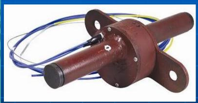
n FBG roof displacement sensor,
