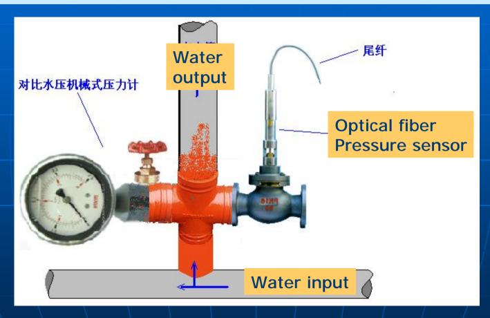
nIllustration of water pressure measurement using fiber optic pressure sensors.
