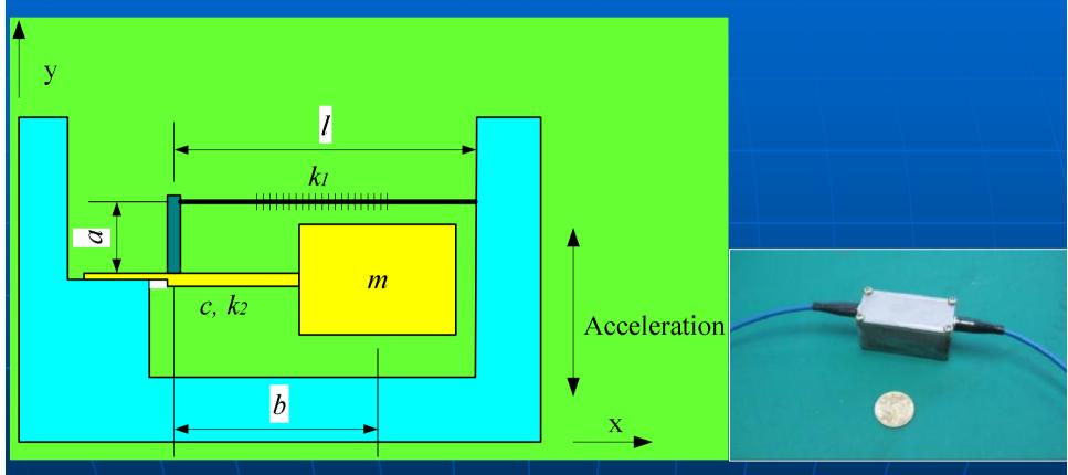
nCantilever based accelerometer:
