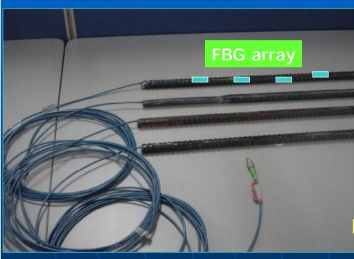
n FBG rock strain sensor array on steel bar
