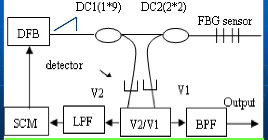
2. SCM PID control to lock the DFB LD to -3dB point in the FBG spectrum.
