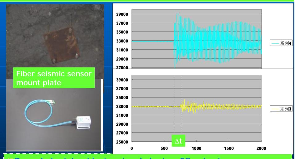
nRecorded mining blaster signals by two FO seismic sensors located 170 m apart. The time delay is apparent which can be used for seismic source location.
