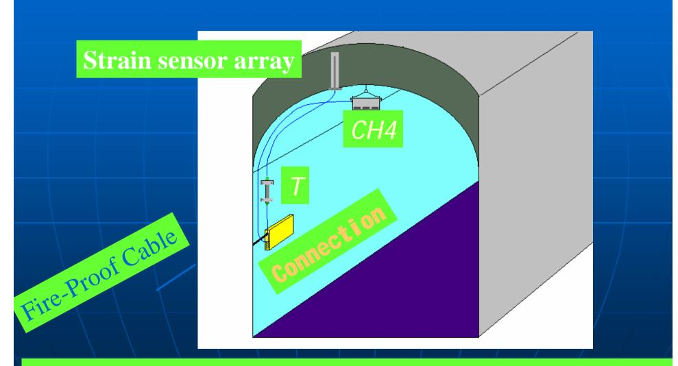
Illustration of Fiber Optic Sensor Installation in the Mine.
