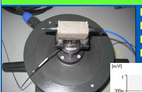
n Sensitivity: 0.1mg; n Range: 0-10g. n BW: 3-400 Hz nAuto-drift compensation
