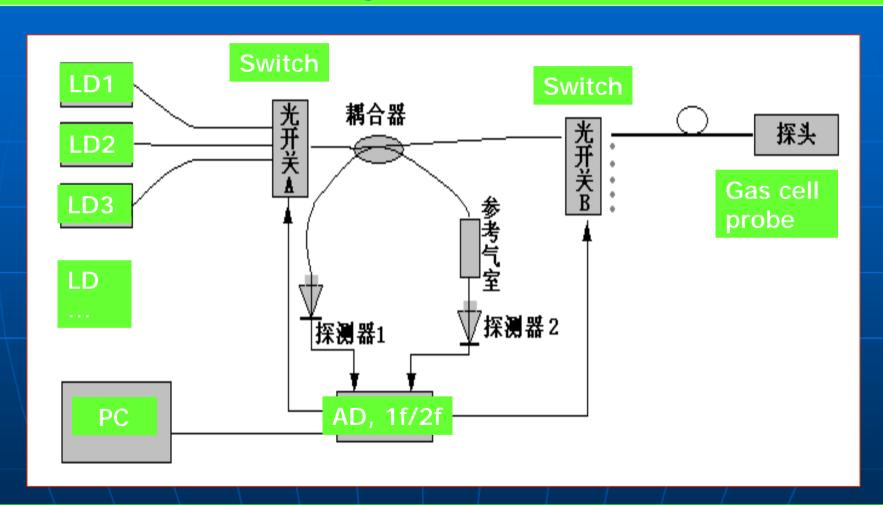
nOne gas cell addressed by a bank of laser diodes, which emits at n absorption band of the gases to be monitored.
