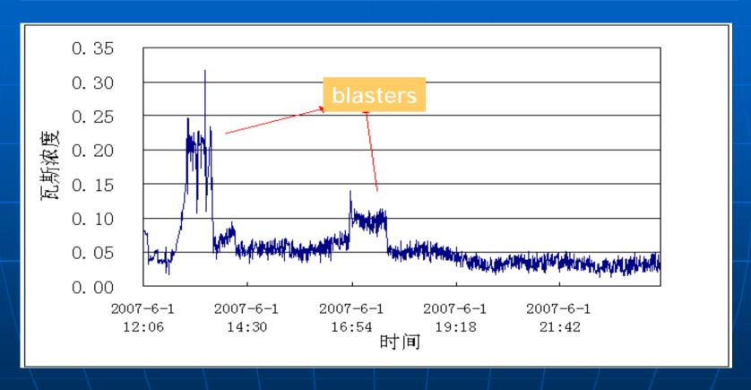
nRecord of methane gas concentration change with time (increase of concentration can be observed after blaster events which agrees with the conventional sensor data).
