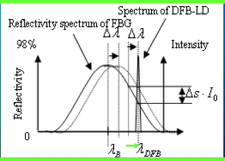
nFBG edge to give acceleration signal; nPID LD current lock to track FBG slow drift.
