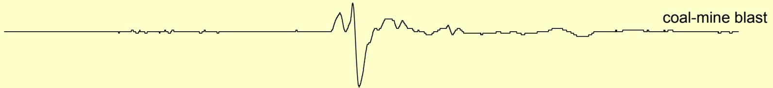
Airblast is a pressure wave time history that creates a push (positive pressure) and pull (negative pressure) effect. For simple time histories, frequency can be determined with the same methodology as used for ground vibrations.
