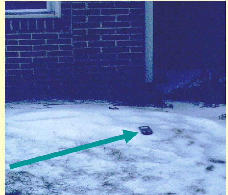
Location relative to the structure. Sensor placement should ensure that the data obtained adequately represents the vibration levels received at the structure being protected. The sensor should be placed within 10 feet of the structure or less than 10% of the distance from the blast, whichever is less .
