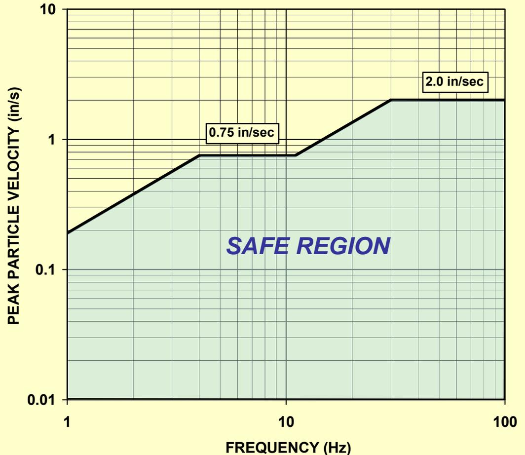
Figure 1.—Modified Blasting Level Chart
