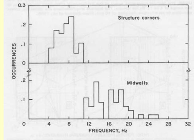
FIGURE 14. Natural frequencies of homes as reported in USBM RI 8507 (Siskind et al., 1980b). Corners represent racking of whole-structure response, and midwalls represent membrane-type flexure with associated secondary noises and rattling. The lighter and more flexible walls have higher natural frequencies and relatively large motions.
