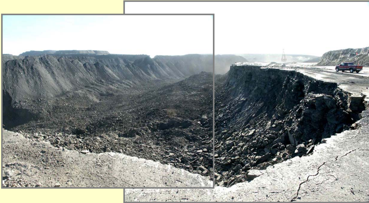
Composite photograph showing typical fragmentation distribution from a well-timed coal-casting shot.
