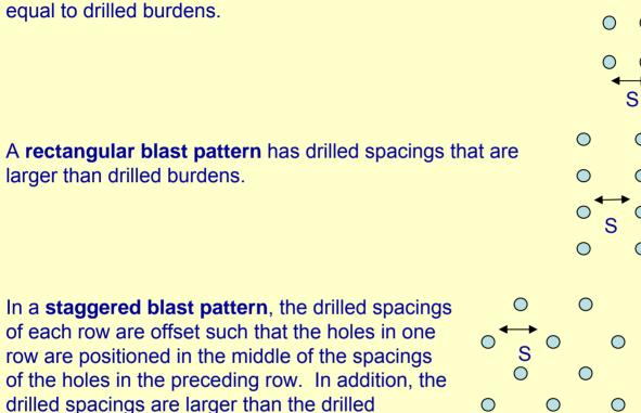
A square blast pattern has drilled spacings that are
