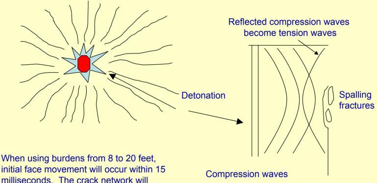
milliseconds. The crack network will establish and rock movement will begin after 1 millisecond per foot of burden on the hole.
