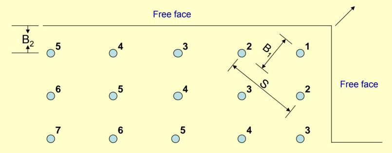
Numbers indicate firing sequence ( $B_1$  = true burden;  $B_2$  = apparent burden).\*
