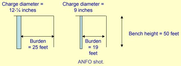
\*Note that both these assumptions with respect to charge diameter are first approximations. A blaster can modify the charge diameter:burden ratio based upon his or her experience and knowledge of the explosive being used, the rock type, and the specifics of the operation.
