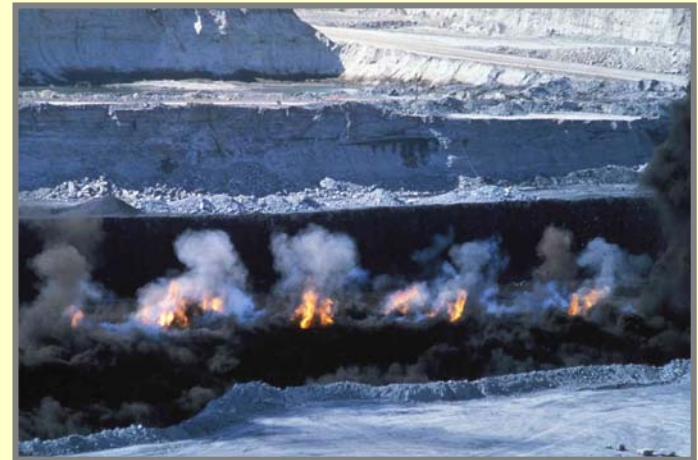
Detonating cord used to fragment coal.
