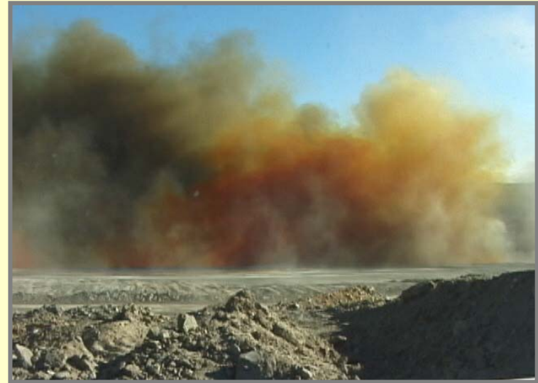
Nitrogen oxides ( \text{NO}_x ) form dark brown fumes after a coal-mine cast blast.
