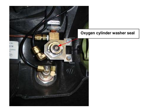
4. Prior to donning, OPEN the oxygen cylinder. Does the alarm and TRIM light function properly? Did you hear the alarm for approximately 10 seconds and see the RED, GREEN, BLUE LIGHT SEQUENCE at startup? After start-up did the alarm stop and the TRIM give you a flashing GREEN light? <u>Close the cylinder</u>.
