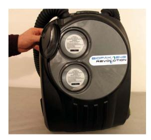
6. Don the Closed Circuit Breathing Apparatus (CCBA). Adjust straps and waist belt to your preference. Attach the face piece to the hose adapter. Ensure the slide is engaged to prevent the adapter from turning.
