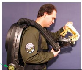
Fully don the CCBA and face piece. Immediately turn on the oxygen cylinder! Fully depress for no more than 2-seconds then release the Emergency By-pass.
