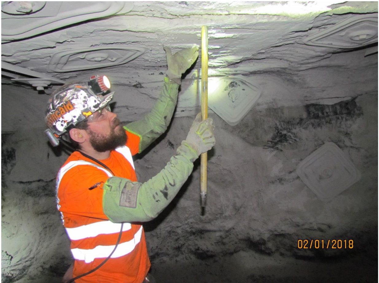
After making a visual inspection, a miner uses the sound-and-vibration method to test the roof.
