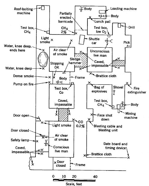
FIGURE 2. - Key Map of Mine Used in Mine Rescue Problem.
