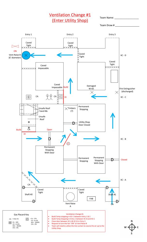
Note: The team may elect to turn the fan "OFF" prior to continuing exploration. In the event the team leaves the fan running and they remove the temporary stopping in XC-C between Entry 1 & 2, they will make a ventilation change without knowing its effects. This ventilation change will move the IDLH across the remaining survivors.
