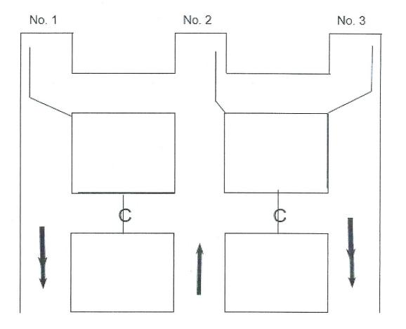
Line curtain required where the continuous miner is cutting or loading coal. Line curtain required in face area where the roof bolting machine is located. Line curtain required to be maintained 10 ft. from the deepest point of penetration.
