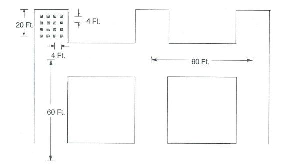
Permanent roof supports to be installed on not more than 4 ft. centers.
