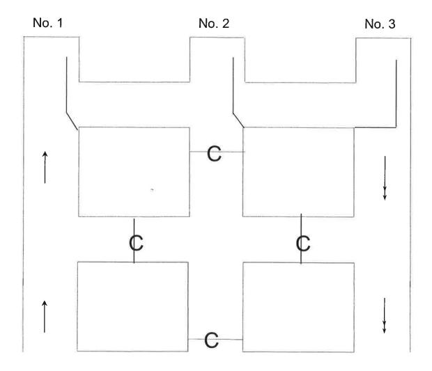
Line curtain required where the continuous miner is cutting or loading coal.
