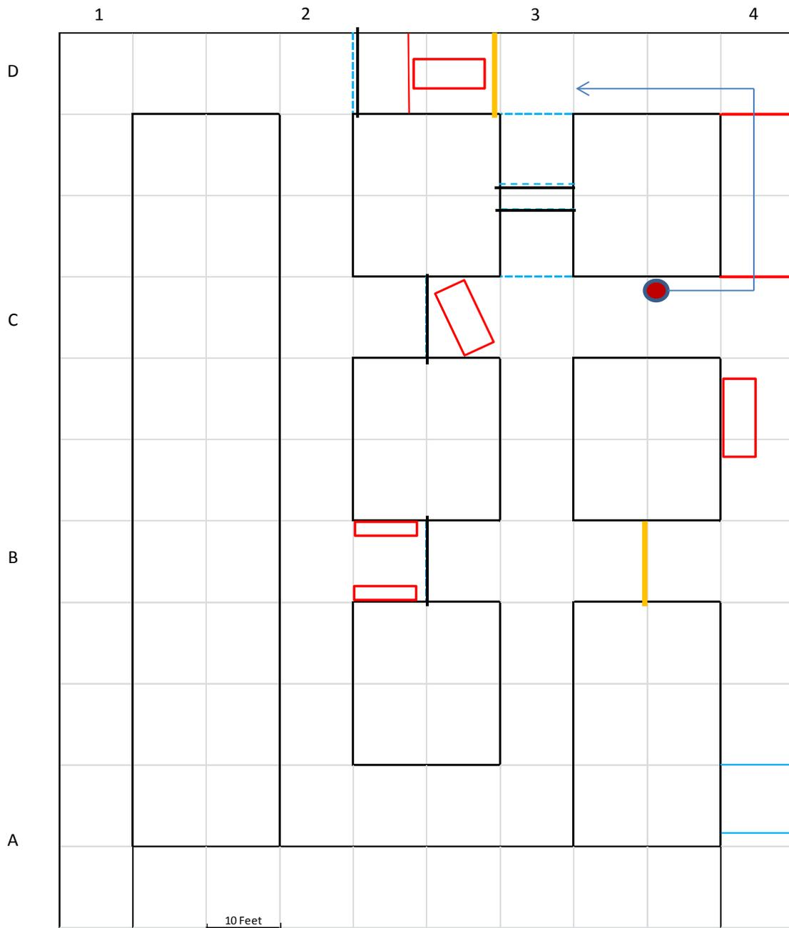
In order to explore behind the barricades for the two missing miners the team will need to ventilate the mine. Ventilation is as simple as sealing the fire, building one stopping and turning on the main, then the auxiliary fan.
