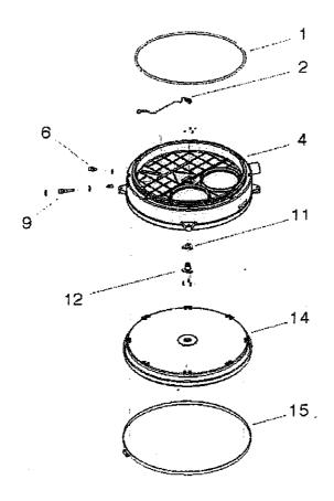
25. Identify Item No.14 A. External DiaphragmB. Diaphragm Disc
