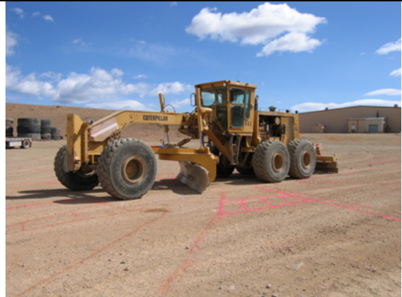
Blind Area Diagram - Motor Grader Ground Plane
