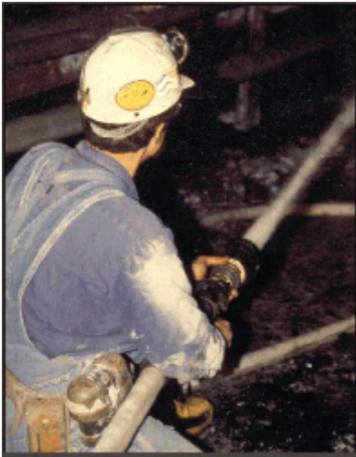
Figure 2.—Measuring the throw distance of water hose.
