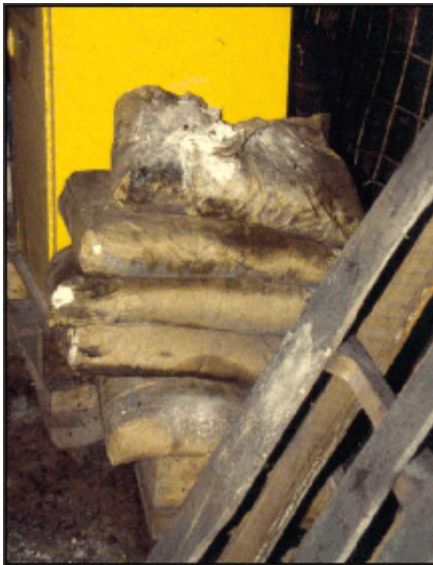
Figure 11.—Rock dust storage unprotected.
