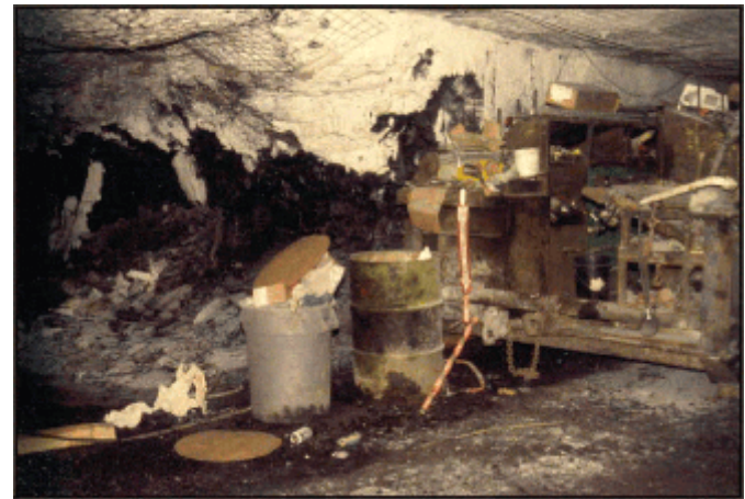
Figure 16.—Improper storage of underground trash.
