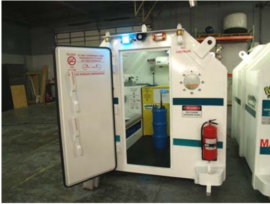
MineARC HRM-08 Steel Refuge Chamber used in study; unit has 8-person design capacity
