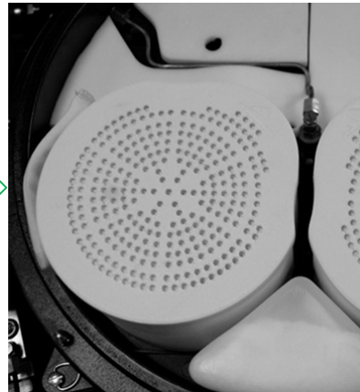
Proper moisture pad installation.
