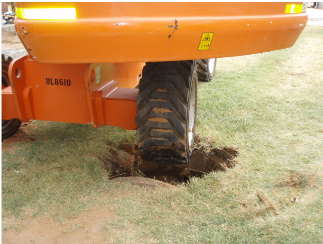
Figure 7 View of boom lift wheel being raised out of soak well.
