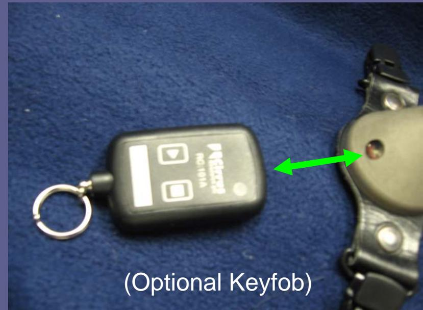
You are now ready to post calibrate the doseBadge and download your data from the doseBadge to the reader. Connect the doseBadge to the reader (align the windows) and press "Calibrate". After the post calibration is complete press the "Read" button. The measurement can now be viewed via the reader display or the dBlink3 software.
