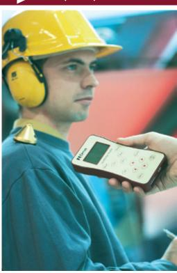
The wireless features of the doseBadge are a significant upgrade to that of traditional style dosimeters, which use a microphone attached to a cable. The primary benefits are:
