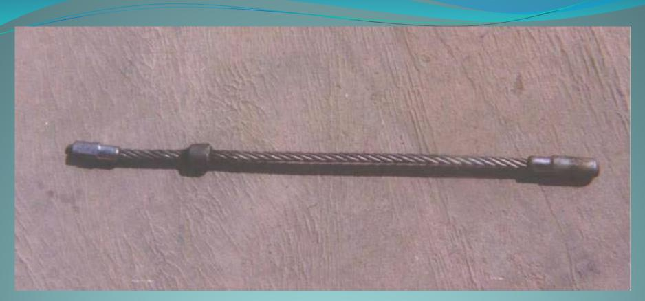
This is a typical source pigtail that is usually secured inside the radiography exposure device or projector.
