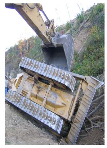
On October 22, 2008, a dozer operator was fatally injured when the dozer he was operating slipped and rolled sideways down a steep 80 foot incline coming to rest on its left side. This was the fourth accident in five weeks where a dozer operator was either fatally injured or suffered serious life threatening injuries. (See Picture to the Left)
