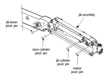
1. Locate and discard all pins in inventory with the following part numbers. Contact Genie's warranty department to receive credit for these pins.
