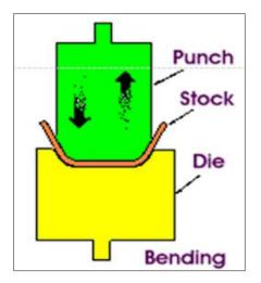
Equipment that uses bending action includes power presses, press brakes, and tubing benders. See Figure above.
