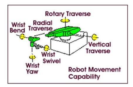
**Servo robots** are controlled through the use of sensors which are employed to continually monitor the robot's axes for positional and velocity feedback information. This feedback information is compared on an on-going basis to pre-taught information which has been programmed and stored in the robot's memory.
