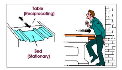
Transverse motion (movement in a straight, continuous line) creates a hazard because a worker may be struck or caught in a **pinch or shear point** by the moving part. See figure to the right.
