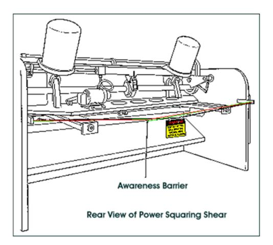
The figure above shows a rope used as an awareness barrier on the rear of a power squaring shear. Although the barrier does not physically prevent a person from entering the danger area, it calls attention to it. For an employee to enter the danger area an overt act must take place, that is, the employee must either reach or step over, under or through the barrier.
