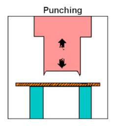
Shearing action involves applying power to a slide or knife in order to trim or shear metal or other materials. A hazard occurs at the point of operation where stock is actually inserted, held, and withdrawn.
