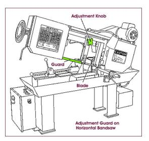
The figure below shows an adjustable enclosure guard on a band saw.
