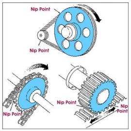
Nip points can occur between rotating and fixed parts which create a shearing, crushing, or abrading action. Examples are: spoked-handwheels or flywheels, screw conveyors, or the periphery of an abrasive wheel and an incorrectly adjusted work rest. See Figure below.
