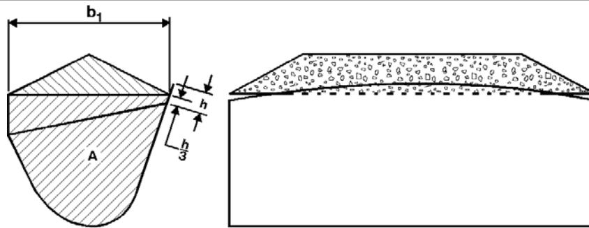
**h = DISTANCE FROM SIDE CUTTING BARS TO FORWARD POINT OF CUTTING EDGE.**
