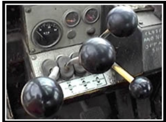
Hard lever handles can lead to contact stress.
