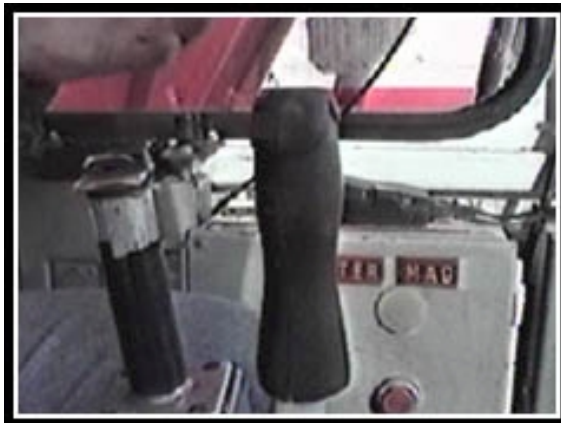
Contoured lever grips are preferred to reduce contact stress and promote neutral wrist postures.
