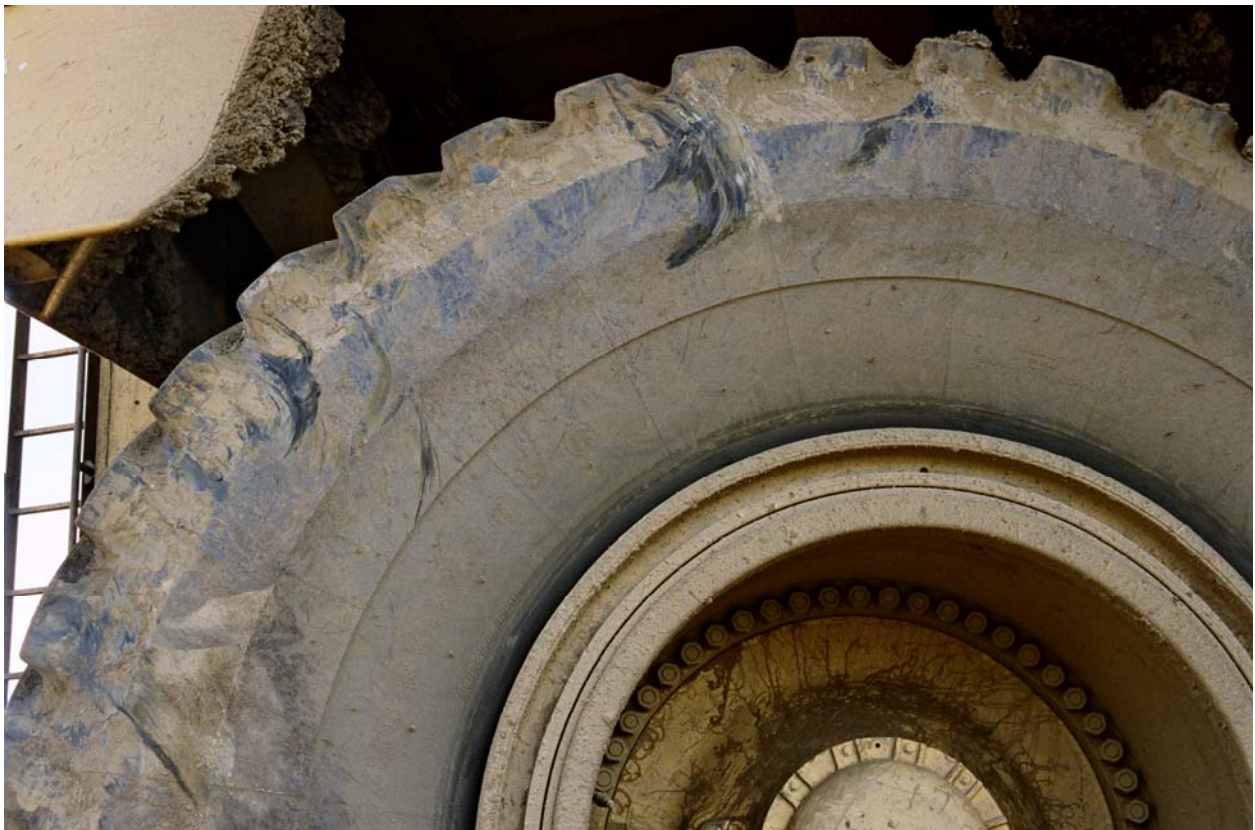
Photograph # 7 Shows marks on the front driver's side tire of the heavy haul truck.
