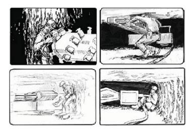
Fatal accident statistics show that the majority of all non-maintenance related crushing accidents involving remote controlled continuous mining machines happened when the victim was located within the turning radius of the machine while it was being trammed.
