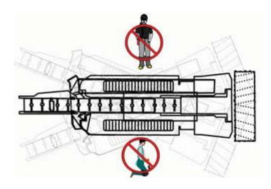
The middle of the remote control continuous miner (pivot point) is not a safe place from which to reposition or tram the machine during a place change.
