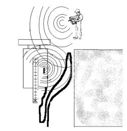
If the remote control continuous miner is not following the commands of the radio remote control, DO NOT get within the machine's turning radius to get closer to the machine's antenna.
