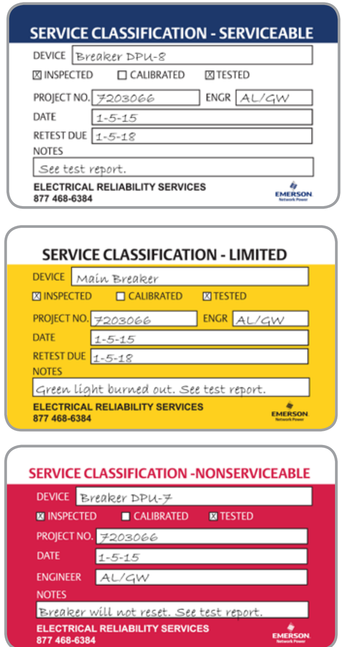
Figure 1. Field testing labels help satisfy documentation requirements of NFPA 70E 2015.
